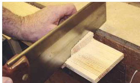
▲ Pic.8 ...is marked out and cut by hand
